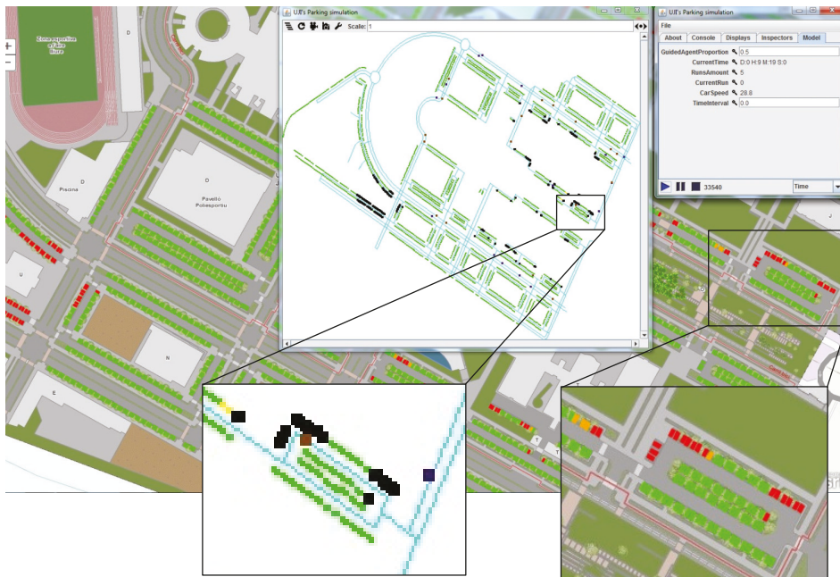
Figure 3. One of the simulator applications running in the foreground, while in the background a web map shows the parking spots' current status as stored in the SPS. In the simulator, black squares represent parked agents. In the web map, red squares represent occupied parking spots.
