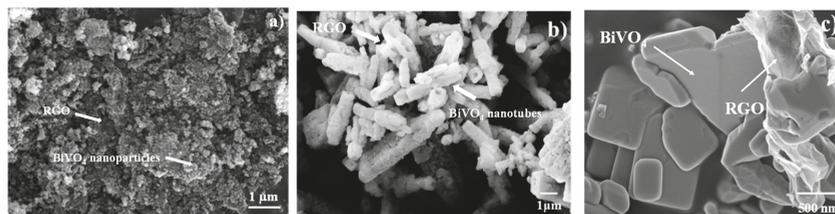
**Figure 1.** SEM images of BiVO<sub>4</sub>/reduced graphene oxide (RGO): (a) BiVO<sub>4</sub> nanoparticles/RGO; (b) BiVO<sub>4</sub> nanotubes/RGO; (c) BiVO<sub>4</sub> nanosheets/RGO.
