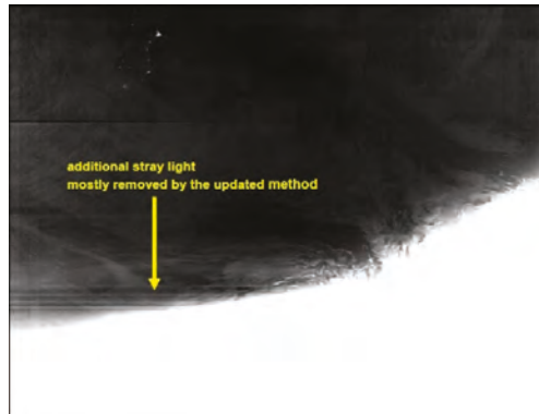
Figure 11. DNB image from October 5, 2013, 5:06 GMT, corrected by the updated method. The residual artifact from additional stray light is significantly reduced.
