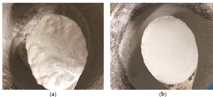
Figure 8. Flow state of ECC mortar. (a) Dosage 3%, w/c 0.24; (b) Dosage 2%, w/c 0.23.
