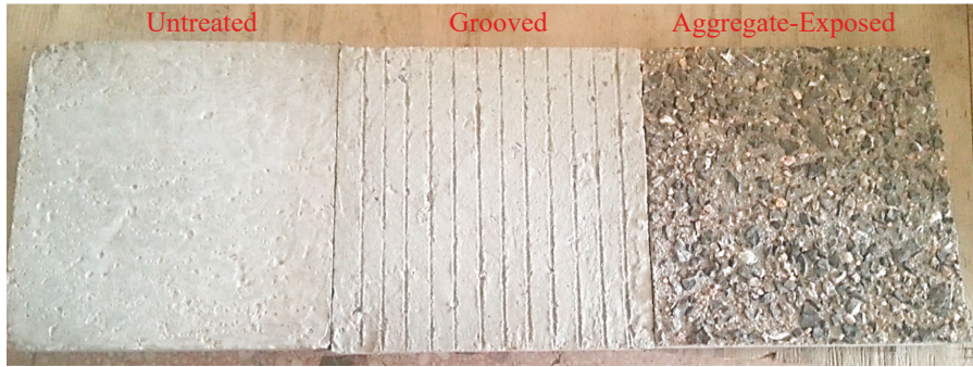
Figure 3. Cement concert slabs with three interface types.
