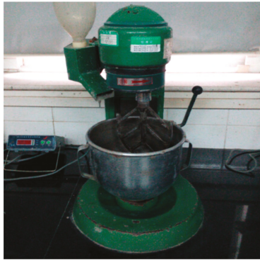
Figure 1. Cement mortar mixer.
