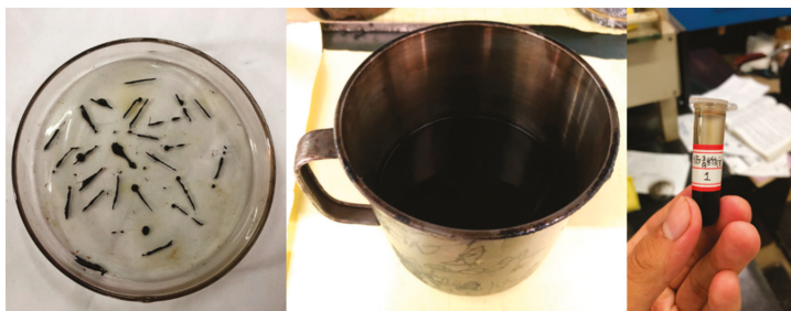
Figure 8. Extraction and storage of asphalt binder coated on Dramix steel fibers.
