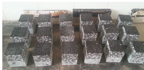
Figure 4. Specimens for the direct shear test with different interfacial treatment.
