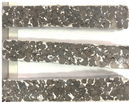
Figure 7. The beam specimens of the SFP materials.
