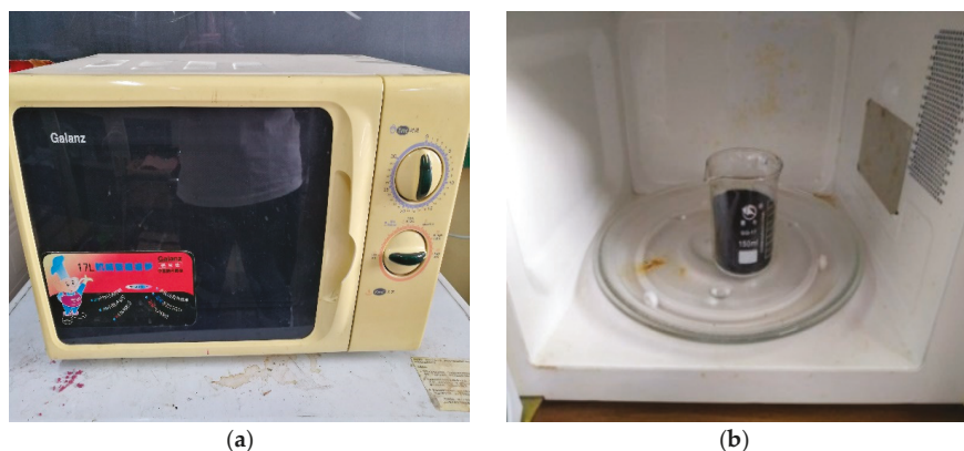
Figure 1. Rubber powder activation equipment: (a) microwave oven and (b) microwave-activated crumb rubber.
