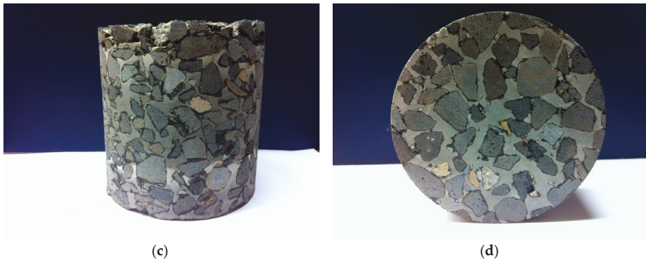
Figure 3. Sample before and after sawing. (a) Sample coring, (b) slab sample after coring, (c) sample before sawing, (d) sample after sawing.
