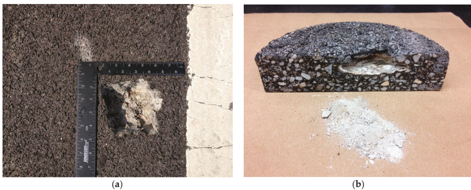
Figure 1. Field observation of clay ball. (a) Opened and cleaned clay ball; (b) sliced core from clay ball area.
