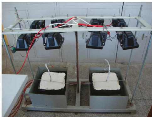
Figure 5. Simulation of solar radiation using an iodine tungsten lamp.
