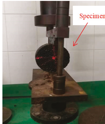
Figure 5. Freeze-thaw splitting test.
