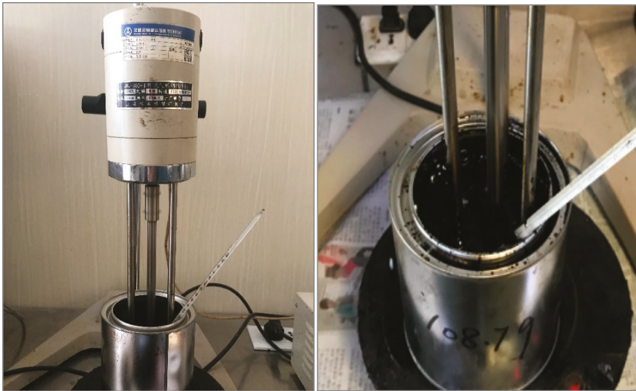
Figure 1. Preparation of HVMA using high-speed shear mixer.
