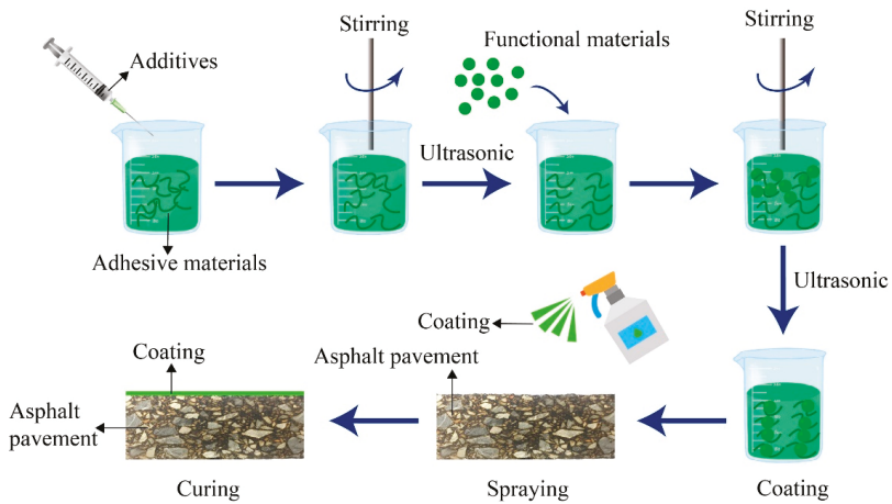
Figure 3. Schematic of the coating preparation process.
