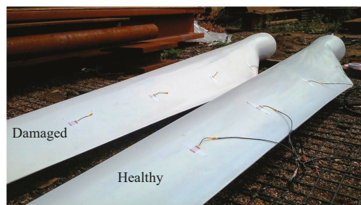
Figure 2. Wind turbine blades (WTBs) with delamination and without delamination in which the guided ultrasound wave tests were applied.
