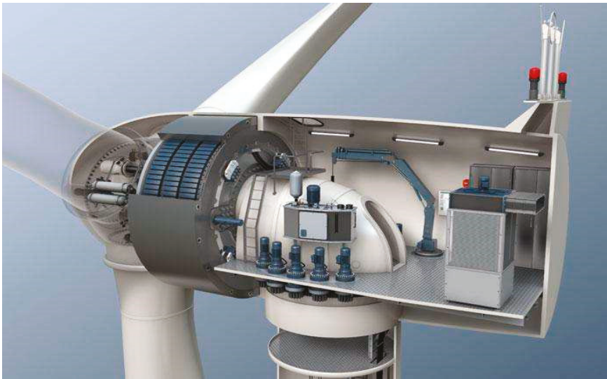
Figure 4. Permanent magnet synchronous generator (PMSG).
