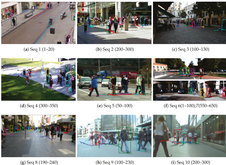
Figure 6. Tracking results on the 2D MOT 2015 dataset. There are ten sequences in the figure, in which (f) contains two sequences. The ETH-Crossing sequence is not shown because it has less targets. The former six sequences (a–e) and the upper one in (f) are static camera cases; the rest are motion camera cases.
