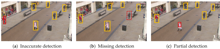
Figure 1. Illustrations of detection failures in three consecutive frames. The solid yellow bounding boxes represent the correct detection responses, and the red boxes are error cases. (a) The red bounding box is a deviation detection that does not exactly match the target. (b) The red dashed bounding box indicates a missing detection. (c) The detection response only includes the upper body of the target.
