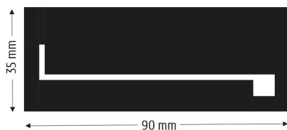
Figure 1. Design of the sputter mask used for patterning the thermocouple leg. The mask is fabricated out of stainless steel and has a thickness of 0.5 mm.
