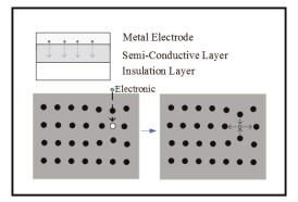
Figure 14. Schematic diagram of electron trapping.
