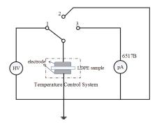
Figure 3. Schematic diagram of thermal stimulation current method.
