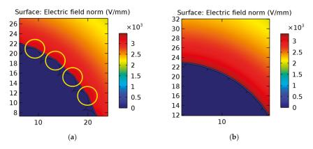
**Figure 10.** Location and magnitude of the maximum electric field for the proposed pliable GIL regarding (a) specimen 2 and (b) specimen 3 of Table 3.
