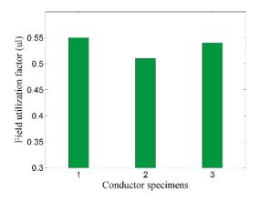
**Figure 12.** Field utilization factor comparison regarding the different conductor specimens described in Table 3.
