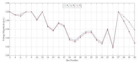
Figure 2. Voltage profile of the load buses for probabilistic multi-objective RPP considering the load demand uncertainty.
