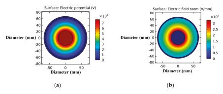
Figure 9. (a) Potential difference and (b) field distribution apropos of the proposed pliable GIL regarding specimen 3 of Table 3.
