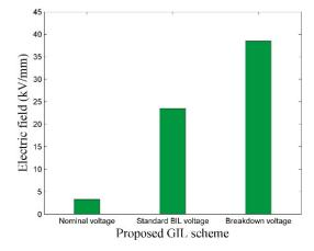
Figure 15. Electric field appraisal for the proposed FGIL scheme regarding operational, standard BIL, and breakdown voltages.
