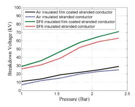
**Figure 20.** Power frequency disruptive discharge investigations regarding air and SF<sub>6</sub> for different FGIL models.
