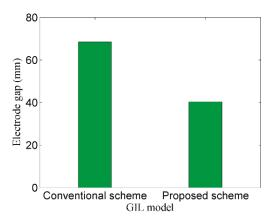
Figure 13. Electrode gap comparison between conventional and proposed flexible GIL (FGIL) schemes.
