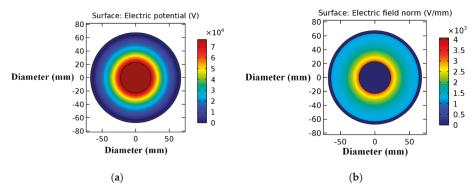
Figure 4. (a) Potential difference and (b) field distribution apropos of the proposed pliable GIL regarding specimen 3 of Table 2.
