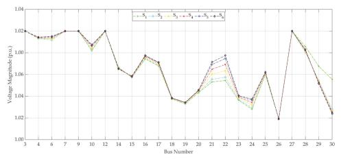
**Figure 3.** Voltage profile of the load buses for probabilistic multi-objective RPP considering the wind power generation uncertainty.
