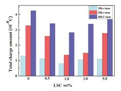
Figure 11. The total amount of charge in the LDPE when the composite with different LSC content acts as a semiconductive layer.
