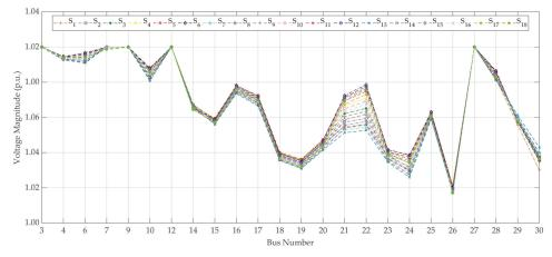
**Figure 4.** Voltage profile of the load buses for probabilistic multi-objective RPP considering the wind power generation uncertainty.
