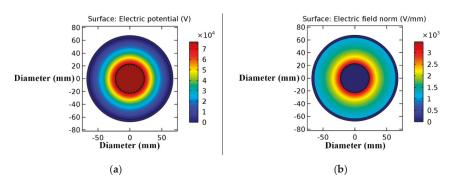
Figure 8. (a) Potential difference and (b) field distribution apropos of the proposed pliable GIL regarding specimen 2 of Table 3.
