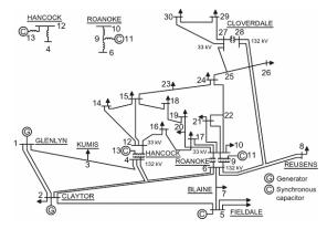
Figure 1. Single line diagram of the IEEE-30 bus test system [43].
