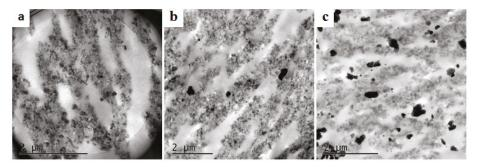
**Figure 7.** Transmission electron microscopy (TEM) micrographs of the semiconductive materials with different LSC contents: (**a**) 0 wt% LSC; (**b**) 0.5 wt% LSC; (**c**) 3 wt% LSC.
