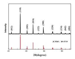
Figure 4. X-ray diffraction (XRD) patterns of LSC.
