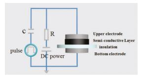
Figure 2. Illustration of the pulsed electroacoustic (PEA) measurement.
