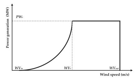
Figure 2. A typical wind turbine characteristic.
