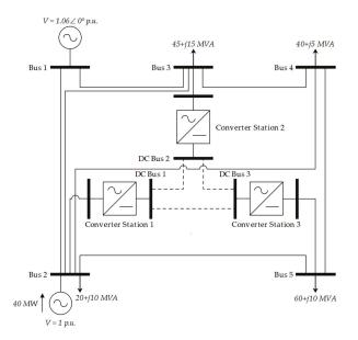
Figure 1. Single-line diagram of a three-bus MT-HVDC system.
