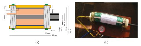
**Figure 17.** (a) Dimensional specifications of the scaled FGIL model and (b) the fully developed scaled FGIL model.
