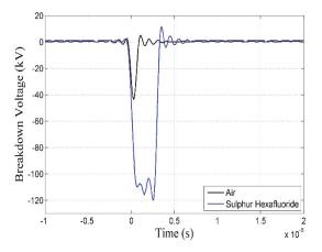
Figure 22. Measured lightning impulse discharge voltage regarding air and  $SF_6$  in fabricated FGIL model at 2.38 bar.
