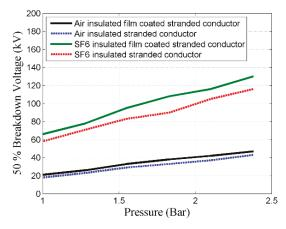
Figure 21. Lightning impulse discharge investigations regarding air and SF<sub>6</sub> for different FGIL models.
