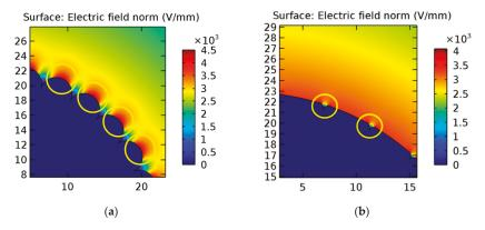
**Figure 5.** Location and magnitude of the maximum electric field for the proposed pliable GIL regarding (a) specimen 2 and (b) specimen 3 of Table 2.
