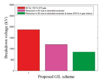
Figure 14. Breakdown voltage (BV) appraisal for the proposed FGIL scheme.
