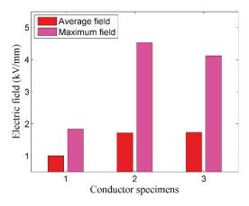
Figure 6. Average and maximum electric field comparison regarding the different conductor specimens described in Table 2.
