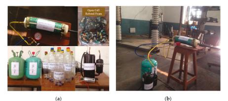
Figure 18. Experimental setup for the dielectric strength testing of the developed FGIL models.
