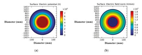
Figure 2. (a) Potential difference and (b) field distribution apropos of a conventional gas-insulated transmission line (GIL) regarding specimen 1 of Table 2.
