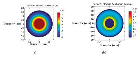
Figure 3. (a) Potential difference and (b) field distribution apropos of the proposed pliable GIL regarding specimen 2 of Table 2.
