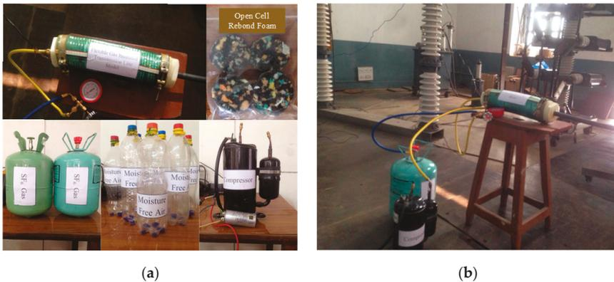
Figure 19. (a) Different components used in the discharge tests and (b) the experimental setup for lightning impulse and disruptive discharge tests.
