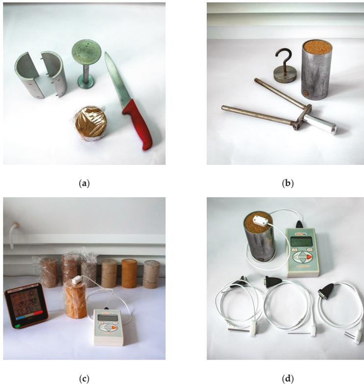
**Figure 1.** Equipment for laboratory testing of thermal conductivity of soil: (a) Metal mold to form cylindrical samples of cohesive soil with a knife and rammer; (b) Steel cylinder with tapping fork that is used to form non-cohesive soil samples; (c) Molded cohesive soil samples during analysis; (d) A set of exchangeable thermal needle probes with KD2 Pro Thermal Properties Analyzer.
