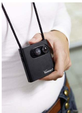
Figure 1. The Microsoft® SenseCam digital camera and how it is worn by participants.
