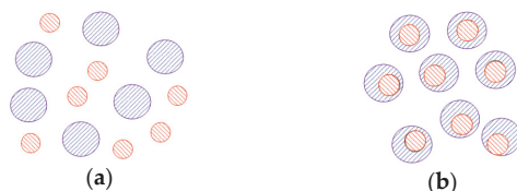
Figure 1. Differences between mixture of two aqueous dispersions of different polymers (polymer 1—blue color and polymer 2—red color) and aqueous dispersion with hybrid particle structure composed of the same two different polymers. In the mixture of two dispersions (a) synergistic effect is much less probable than in dispersion with hybrid particle structure (b) [4].
