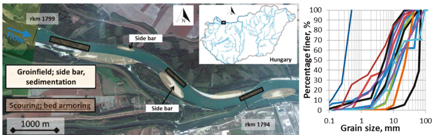
Figure 1. The sketch of the investigated Danube study reach (left) and grain size distributions taken from the investigated reach (right). The characteristic water discharges are mean flow Q_m = 2000 \text{ m}^3/\text{s} , range of bankfull discharge Q_{bf} = 4300\text{--}4500 \text{ m}^3/\text{s} , 2, 10 and 100-year flood event Q_2 = 5950 \text{ m}^3/\text{s} , Q_{10} = 7950 \text{ m}^3/\text{s} and Q_{100} = 10,400 \text{ m}^3/\text{s} [23].
