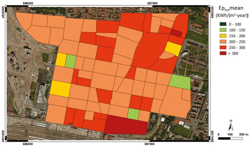
Figure 5. E_{p_{tot}} mean value map corresponding to the validation area (Bolognina) at block scale. Bing aerial imagery is used as the base map.
