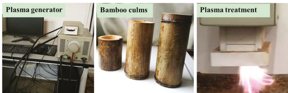
Figure 1. The plasma treatment of bamboo culms using a plasma generator.
