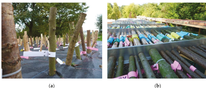
Figure 2. Field tests with sapling wood specimens. (a): in-ground exposure. (b): specimens with and without bark, partly wrapped with a cotton sponge.
