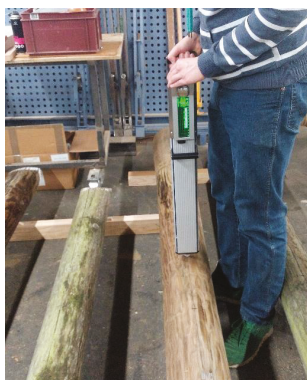
Figure 2. Drilling-resistance measurements in a preservative-treated pole.
