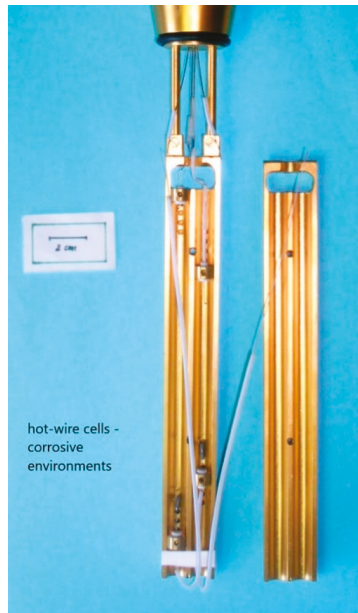
Figure 3. TiN film protection of TWH instrument for humid air measurements—detail of hot-wire cells. Hot-wire was made from tungsten (diameter 8.94 \pm 0.05 \mu\text{m} , long wire length 148.92 \pm 0.02 \text{ mm} and short compensating wire length 71.69 \pm 0.02 \text{ mm} ). The global uncertainty of the measurement, at a 95% confidence level, was estimated to be U_\lambda = 1.7\% . Adapted from [35].
