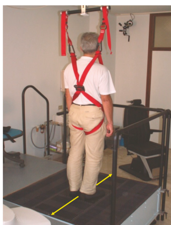
Figure 1. This shows a platform that can produce movements of the supporting base in various directions in the horizontal space according to different driving functions.
