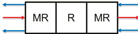
Figure 12. Proposed redesign of the polymer membrane reactor with membrane being removed from the center of the unit (MR = polymer membrane reactor, R = Reactor).
