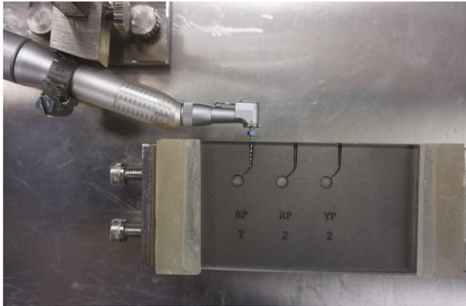
**Figure 2.** CF testing device illustrating positioning of dental handpiece, NiTi rotary instrument, and stainless steel block.
