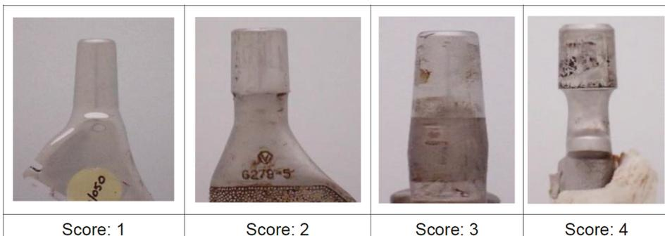
Figure 1. Corrosion damage scores of 1 through 4 for stem tapers.
