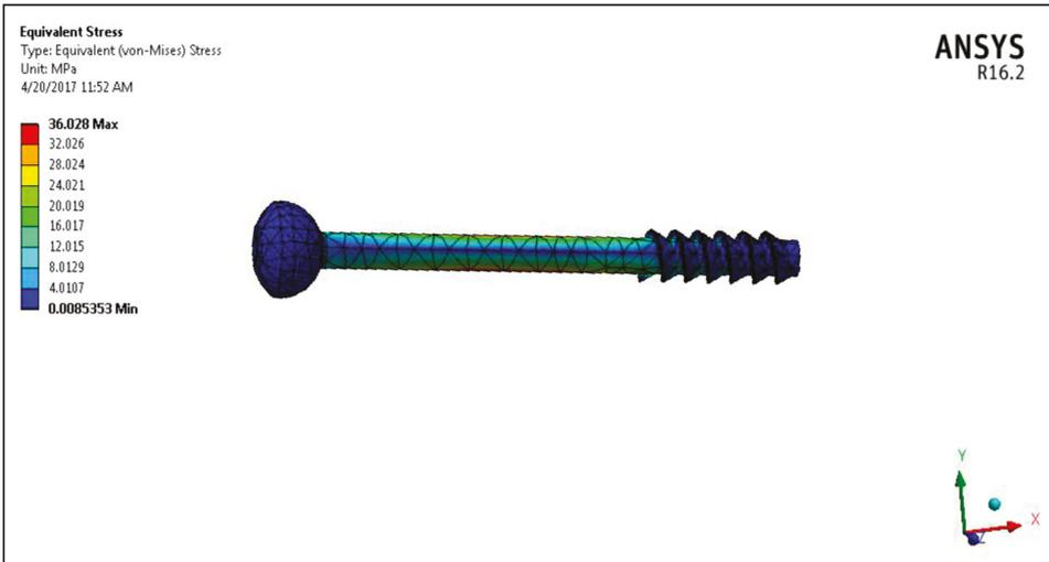
Figure 14. The von-Mises stresses in the cannulated screw.
