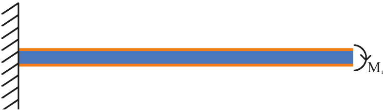
Figure 3. Piezoelectric action (PIN force model).
