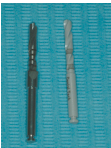
Figure 1. Macroscopic aspect of the steel drill (left) and zirconia drill (right) used in the present study.
