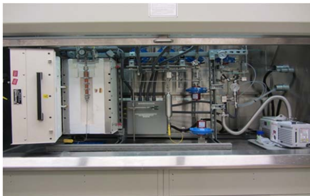
Figure 23. High-temperature reactor installed on PNNL's Sievert's system for measuring isotherms and for life cycle testing of metal hydride thermal energy storage materials.
