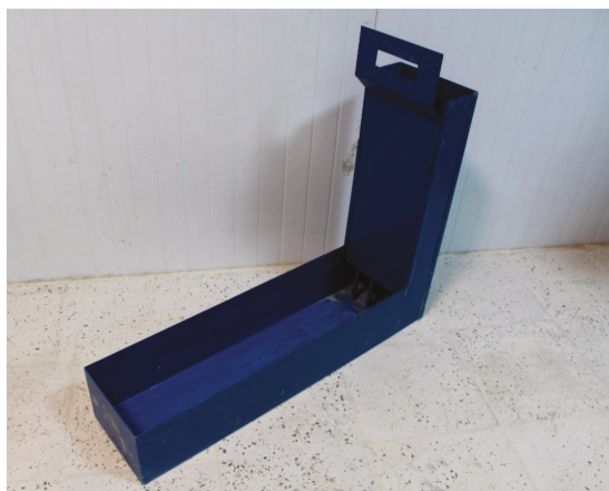
Figure 8. The L-box setup for workability measurement.
