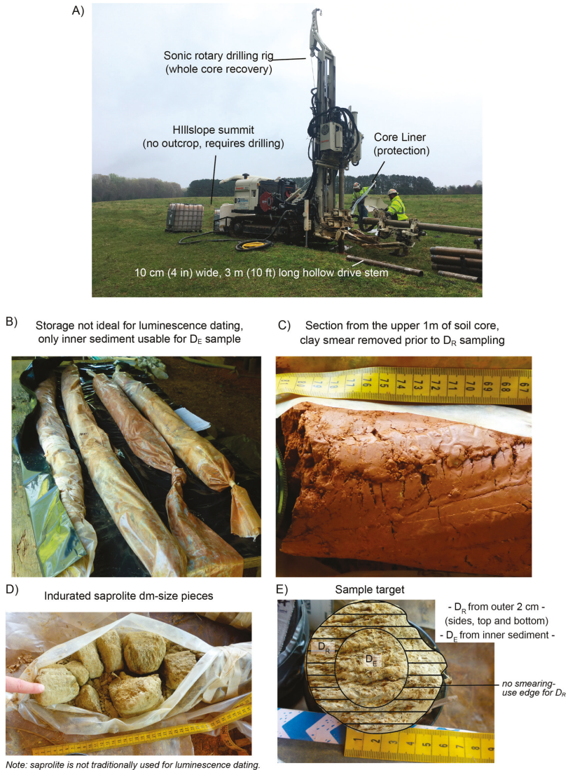
Figure 5. (A) Sonic-rotary drill rig at hillslope summit. Photo credit: Martha Eppes. (B) Yield, including intact soil and saprolite cores that were stored in plastic liners and outdoors. While not ideal, these conditions are not an impediment to luminescence geochronology [22]. (C) The upper 1 m of core shows signs of sediment and soil smearing on the sides, this material should be removed prior to dose rate sample collection. (D) Indurated saprolite, no smearing. (E) The dose rate sample will include the outer 1–2 cm from the sides, top, and bottom of the sample section. The inner most material is used for the equivalent dose sample.
