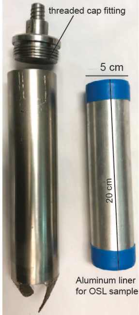
Figure 2. Shallow-sediment auger set-up for luminescence sampling. (A) Optically stimulated luminescence (OSL) auger head with T-shaped handle. The enclosed OSL auger head is fitted with an aluminum liner to contain the OSL sample in a light-proof tube. (B) T-shaped handle with extension rods are used to drive bucket auger. (C) Each drive requires sediment removal from hole, placed on the surface in stratigraphic order (by depth) until desired OSL sampling depth is reached. This material may be needed as part of the D R sample.
