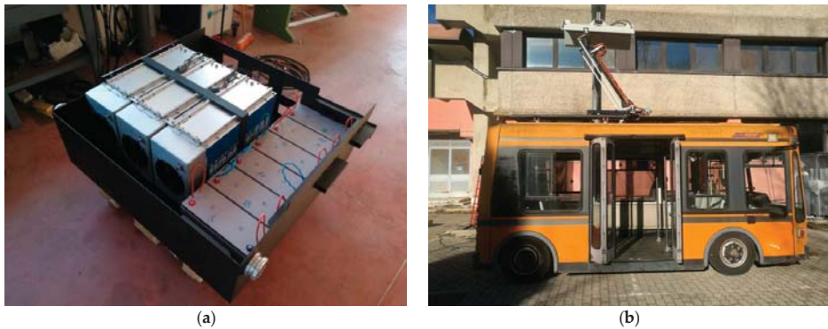
Figure 1. (a) Hybrid Storage system on board the bus; (b) and the pantograph for ultrafast charge.
