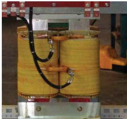
Figure 3. Inductor used in the charging station.
