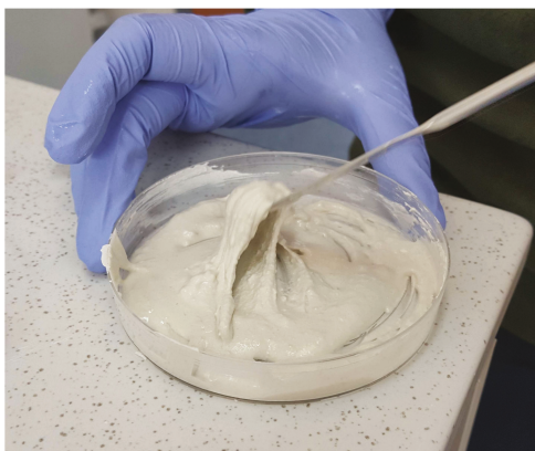
Figure 3. Chewing gum-like consistency of P50 samples after mixing of bioceramic and polymeric components.
