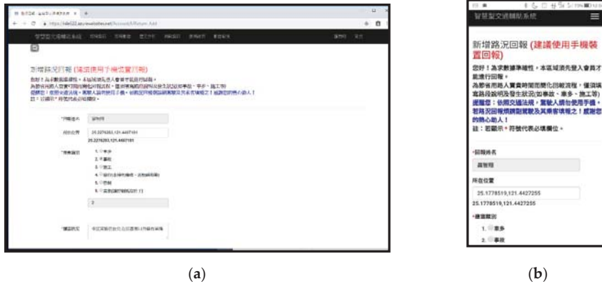
Figure 14. Road condition user reporting function displays for (a) computer and (b) mobile phone. After logging into the system, when a user arrives at an accident emergency site, their intelligent handheld device can read the longitude and latitude of their location through the built-in GPS function, and present it in real time on the reporting page to complete add road condition reporting information.
