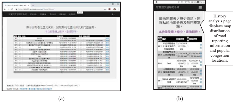
Figure 15. History analysis page displays map distribution of road reporting information and popular congestion locations for (a) computer and (b) mobile phone. History analysis page of the system will obtain the return information through the cloud database; that is, clicking on the navigation function of the page will open the icon of the Google Maps display endpoint and go there.
