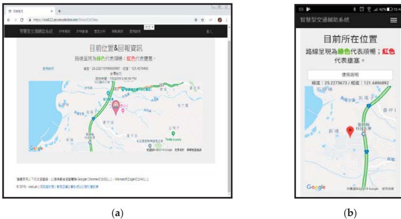
Figure 8. Real-time traffic information displays for a (a) computer and (b) mobile phone. In this step we take the longitude and latitude of the user's location and present it on a map through the GPS function of the intelligent handheld device held by the user, and then, display the "real-time status" data, such as the green color indicating the smooth conditions and red indicating congested road conditions.
