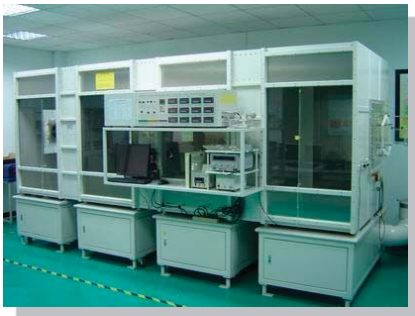
(a) Testing workbench with a wind tunnel
