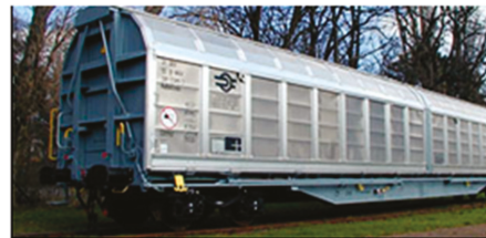
Figure 6. Habis wagon and its characteristics.
