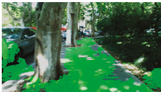
Figure 11. An example of expansion error. The ground has been unexpectedly expanded to a part of the car.
