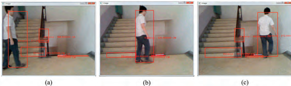
Figure 26. The detection of static and dynamic obstacles. (a) Walking people walks from the left side; (b) Walking people at the middle; (c) Walking people walks to the right side.
