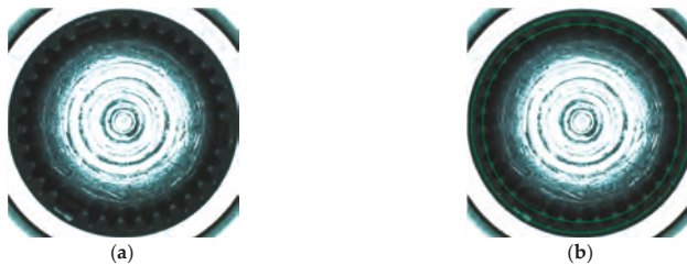
Figure 12. Fitting the spline circles by CAM: (a) Image of spline; (b) Detection results of inscribed and circumscribed circles of spline (denoted by green circles).
