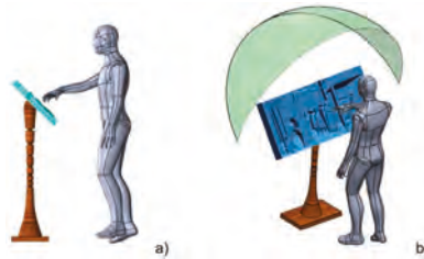
Figure 7. (a) CAD model of the bas-relief and the user; (b) CAD model of the plausible region (green) to host the Kinect®.
