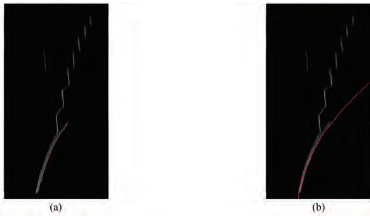
Figure 6. The ground curve in V disparity map. (a) Segment consisting of points (red); (b) The line of the equation (red).
