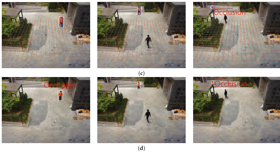
Figure 10. Results of occlusion detection three selected frames in each video: (a) occlusion by background; (b) occlusion by another object; (c) result of occlusion detection in another video and (d) result occlusion detection without depth information.
