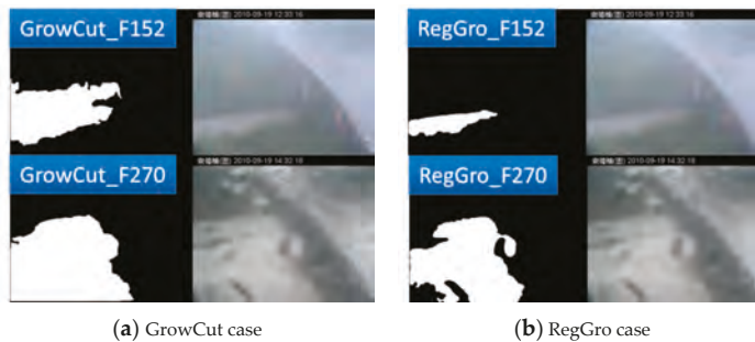
Figure 18. Comparison of the two algorithms with example images from the start (Image 152) and middle (Image 270). (a) GrowCut covering the stains (Image 152) and overestimating them (Image 270); (b) RegGro identifying the flood region (Image 152) and affected by stains (Image 270). (Note: The Traditional Chinese in header of all images is represented the location in the Changed Bridge).
