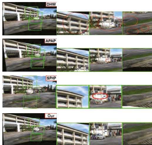
Figure 6. Comparisons among dual homography warp (DHW) [6], as-projective-as-possible (APAP) [18], Shape-Preserving Half-Projective (SPHP) [28] and Our algorithm, Red circles highlight errors.
