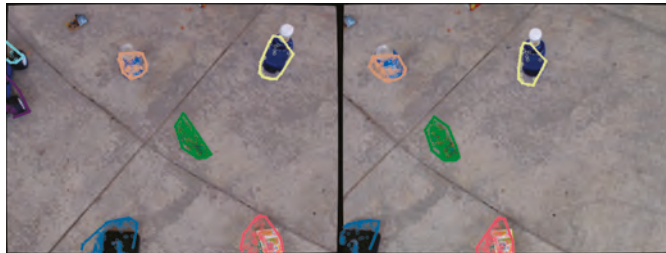
Figure 7. Reprojection of the points belonging to candidate objects, surrounded by a convex hull.
