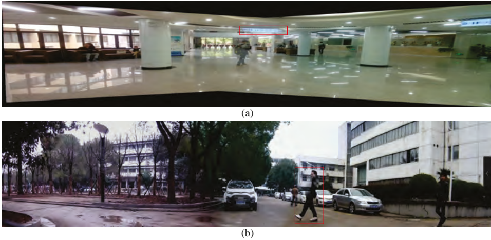
Figure 1. The main reason for ghosting comes from misalignment error. Here we show two types of ghosting in red boxes: (a) ghosting caused by using a global projective warping; (b) ghosting caused by persons moving across seams.
