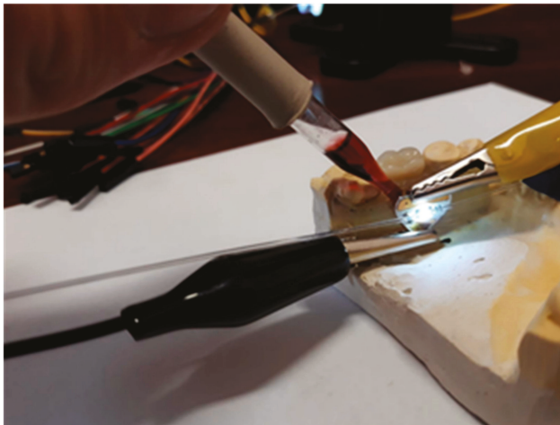
Figure 13. Illustration of the intra-oral optical sensor test procedure for wine color analysis, which assumes having the sensor integrated into a mouthguard and mounted onto a custom jaw mold.
