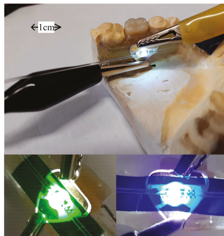
Figure 8. Test setup for the assessment of the point intra-oral sensor spectral attenuation measures: (a) schematic diagram, (b) practical realization with external LED supply and optical filter foils.
