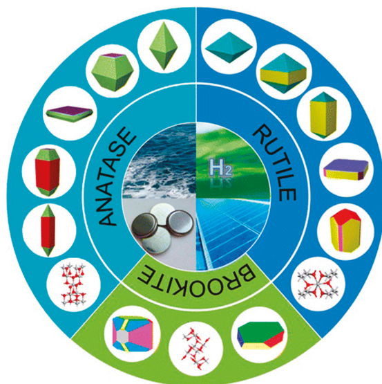
Figure 14. Summary of main shapes and applications (i.e., lithium ion batteries, photocatalytic hydrogen evolution, photodegradation, and solar cells) of anatase, rutile, and brookite TiO 2 crystals with their surfaces consisting of different Facets [89]. Copyright 2014 American Chemical Society.
