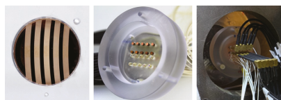
Figure 7. Images showing left—rear of the target mounted in the lexan plate, center—back of the diagnostics package showing the LN pins (top two rows) and PDV probes (bottom two rows), right—rear of the target and diagnostics assembly mounted in the gas gun.
