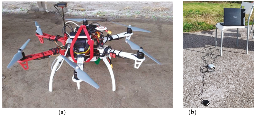
Figure 1. M-UAV radar imaging system: (a) hexacopter with onboard equipment; (b) ground-based GPS station.
