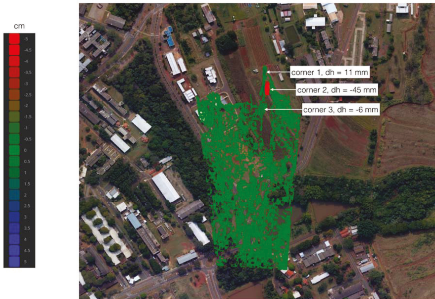
Figure 4. Deformation map of the interferogram 1 and 2—from the first and the second flights. Displacement is positive ( dh > 0 ) when terrain height decreases with time. The coherence threshold is 0.6. Corner reflector 2 was lifted 4 cm in the second flight. The measured displacement was -45 mm.
