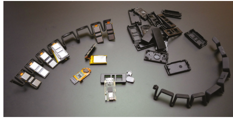
Figure 2. Myo armband tear-down [46].
