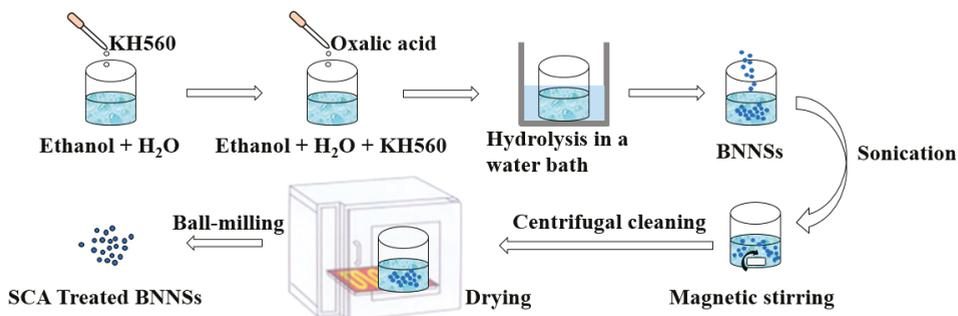
Figure 4. Silane coupling agent (SCA) treatment process.
