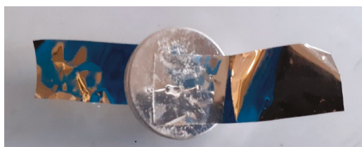
Figure 13. Image of an individual coin cell with welded connections prepared to be tested.
