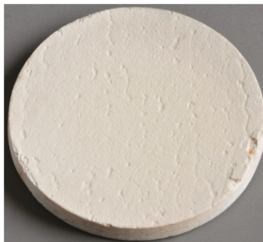
Figure 9. Photograph of VLPPS YAlO_3 coating on FW12 after 1010 cycles of burner rig testing.
