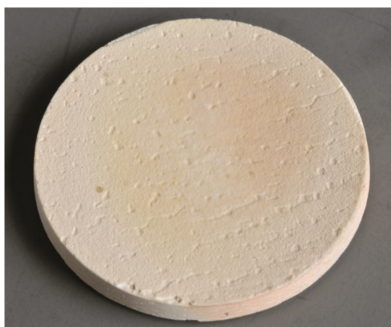
Figure 11. Photograph of VLPPS \text{YAlO}_3 coating on FW 12 after 274 cycles in CMAS test rig.
