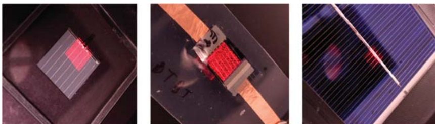
Figure 3. The three samples used in this work, with a random pattern for compressive sampling projected on them. On the left is the c -Si reference cell, in the middle is the organic photovoltaic (OPV) device, and on the right is the large mc -Si cell.
