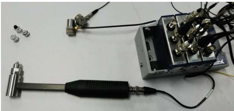
Figure 9. Data acquisition module for collision experiment.
