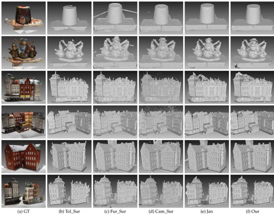
Figure 10. Result of the five methods on MVS dataset [2]. GT is the reference model; Tol is Tola et al. [27]; Fur is Furukawa and Ponce [29]; Cam is Campbell et al. [24]; Jan is Jancosek and Pajdla [5]; Our is the proposed method; and *_Sur is the surface generated by poisson surface reconstruction method [30].
