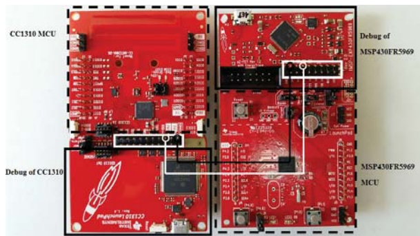
Figure 3. Board configuration for measuring energy use.
