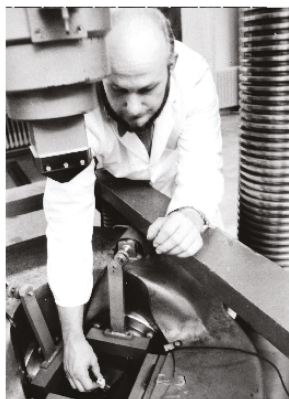
Figure 6. Sample insertion at the triaxial press.
