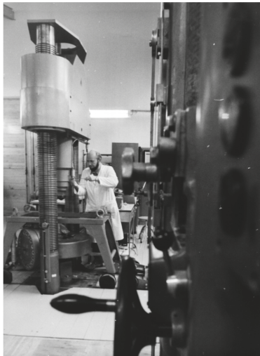
Figure 5. 600 t press with triaxial device.
