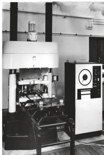
Figure 13. New 400 t press.
