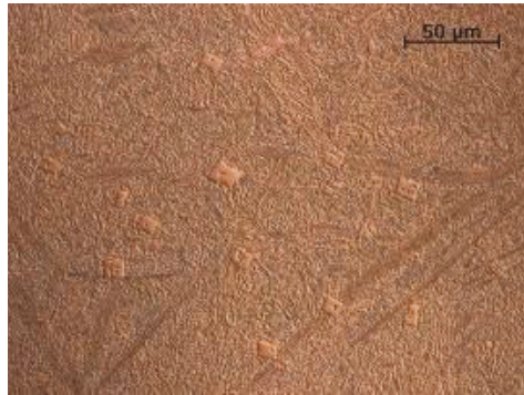
Figure 9. Microstructure of a nanocrystalline layer with carbide precipitates of NANO (Fe-Cr-Nb-B).
