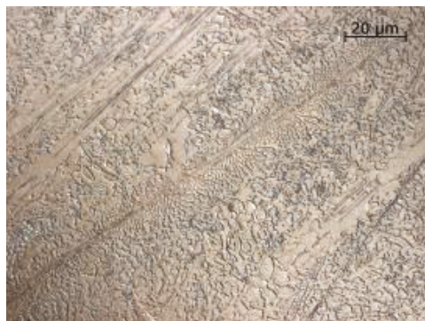
Figure 8. Microstructure of a nanocrystalline layer with eutectic like carbides of NANO (Fe-Cr-Nb-B).
