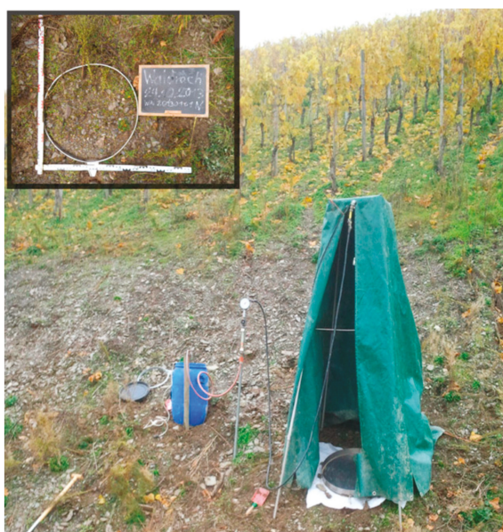
Figure 2. Rainfall simulation experiment: Pump is submerged in a blue water reservoir. Flow control by flow-meter and manometer. The image in the upper left corner shows circular plot. (Images by J. Rodrigo-Comino).
