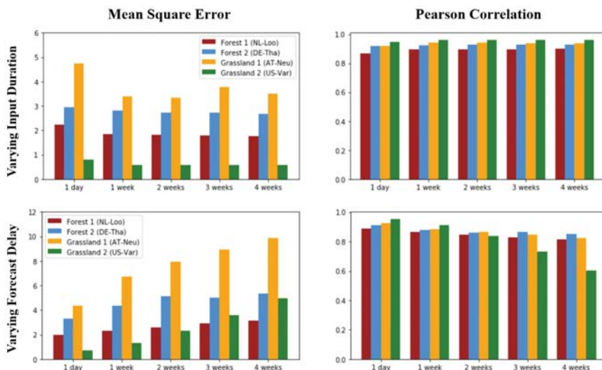
Figure 2. The past-history dependency and GPP forecasting ability of the LSTM model. Upper panel: predicting the current GPP using varying length of historic data on climate drivers. Lower panel: predicting the GPP on varying days ahead in the future using the same two-week length of historic data.
