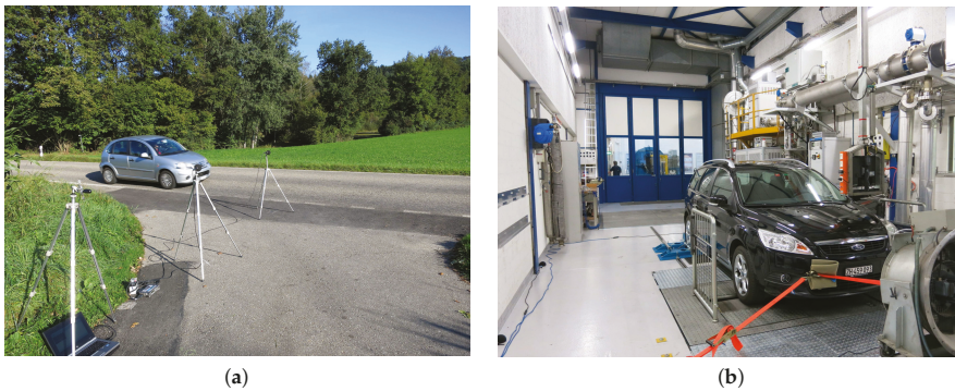
Figure 8. Photographs showing the measurement set-ups for tire noise (a) and propulsion noise (b). In (a), the coast-by situation is depicted with two measurement microphones placed at different distances and a camera connected to a laptop; (b) shows the lab with a passenger car on the chassis dynamometer, the airstream fan in front of the car and two microphones on the floor at the left-hand room edge (emission angles \varphi = 60^\circ and 120^\circ ).
