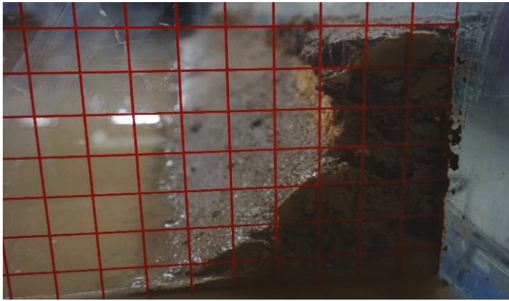
Figure 6. Schematic diagram of a topographical measurement conducted after the collapse section using a system of gridlines.
