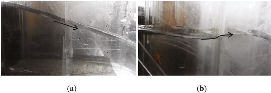
Figure 5. Photograph of water surface: (a) without FGP; (b) with FGP ( \beta = 0.51, \theta = 15^\circ ) (Black arrow stands for the flow direction).
