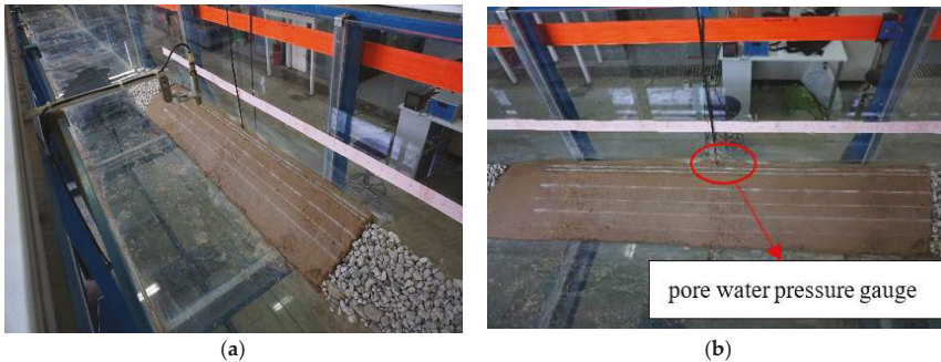
Figure 2. Scheme of the experimental model. (a) Constructed bank slope fitted within the experimental flume; (b) Position of the pore water pressure gauge embedded inside the bank.
