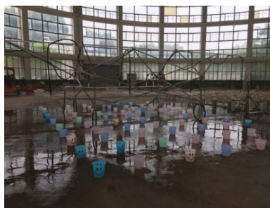
Figure 7. Test plot for the LMIS mobile water distribution.
