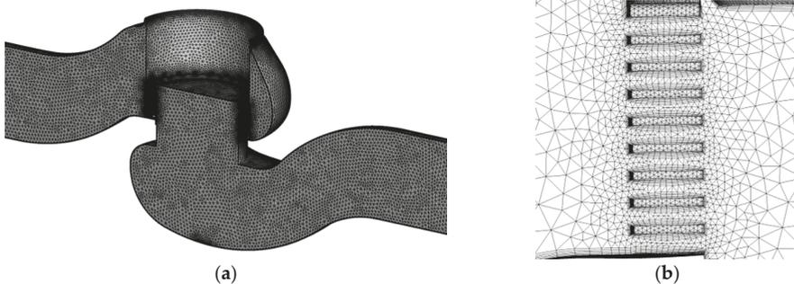
**Figure 2.** Mesh of the sleeve regulating valve with maximum valve core displacement of 60 mm (a) overall view; (b) mesh in the sleeve.
