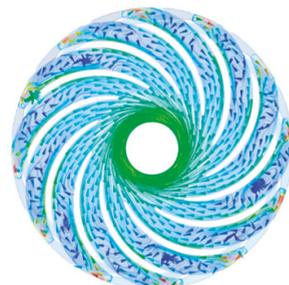
Figure 7. Velocity distribution in the mid-scan of the pump's first stage at different flowrates.
