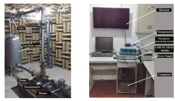
(b) model pump and the layout of the pipelines
