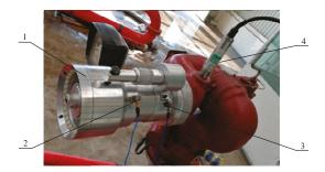
**Figure 18.** The fire-fighting monitor prototype and sensors. The labels are as follows: 1. Fire-fighting monitor 2. Acceleration sensor (three directions), 3. Acceleration sensor (one direction), and 4. Pressure sensor.
