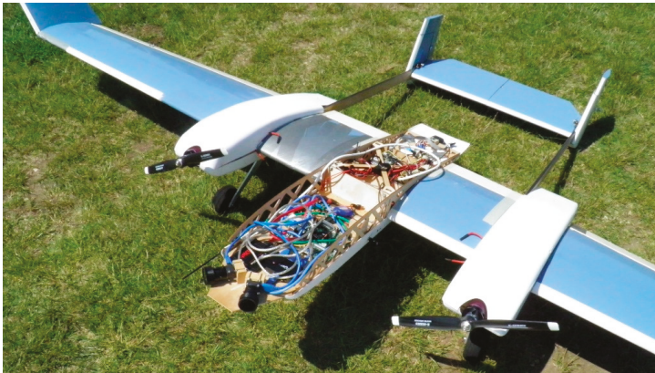
Figure 8. Sindy aircraft with the mounted Nvidia TK1-based visual SAA system.
