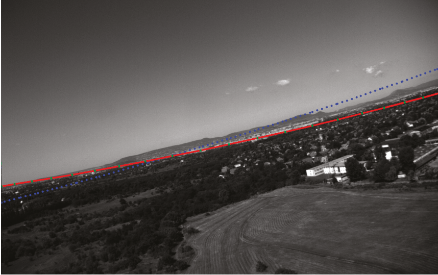
Figure 6. The blue dotted curve represents the pre-calculated horizon. Post-calculated horizon curve is formed by line segments between the green points. The effect of the white urban area under the hills can be seen on the right.
