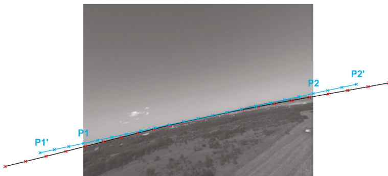
Figure 4. The blue line represents the pre-calculated straight horizon with endpoints P1 and P2. Red crosses and the black curve represent the distorted version of the straight line.
