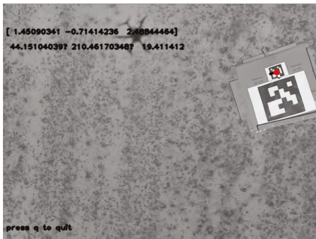
Figure 2. Image retrieved by the Unmanned Aerial Vehicle (UAV) camera after processing using OpenCV/ArUco libraries.
