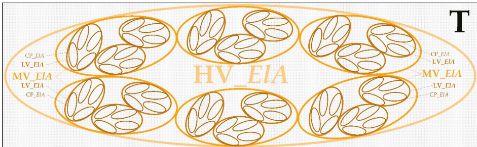
Figure 7. The fractal set of HV, MV and LVGs and customer plants (CP).
