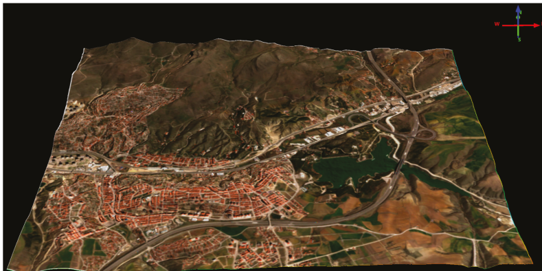
Figure 20. The DTM (digital terrain model) of the study area textured with the Sentinel-2 image.
